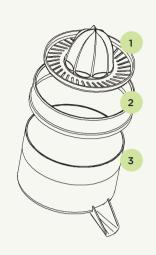
All parts in contact with fruits are removable, which allows a simple and quick cleaning.
